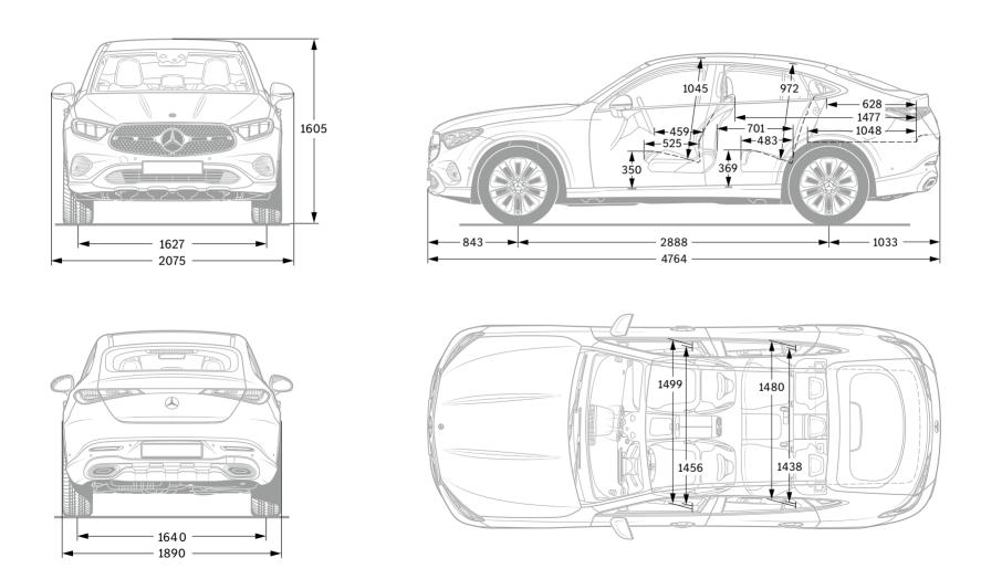
All figures in millimetres. The dimensions shown are mean values. They are valid for vehicles with standard equipment and in unladen condition.
