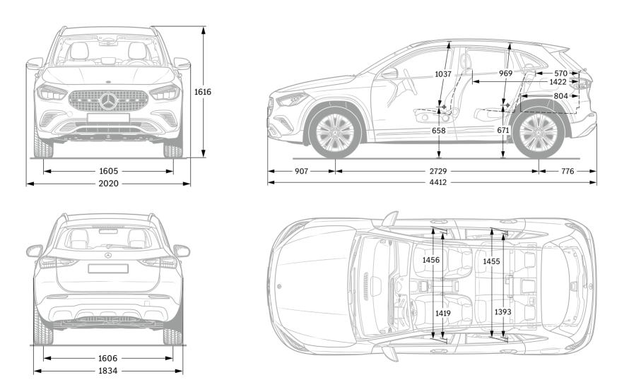
All figures in millimetres. The dimensions shown are mean values. They are valid for vehicles with standard equipment and in unladen condition.
