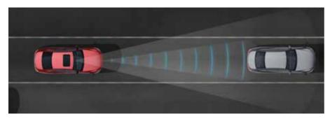
Active Distance Assist DISTRONIC and Active Steering Assist are able to maintain automatically the correct distance to vehicles ahead and to follow them, at speeds of up to 210 km/h.
