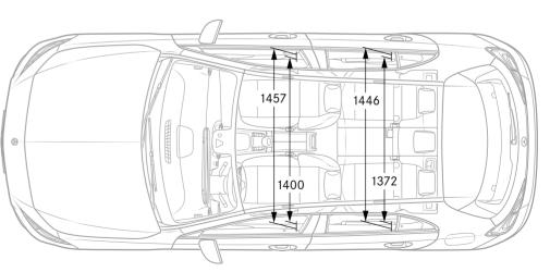
All figures in millimetres. The dimensions shown are average values. They are valid for vehicles in basic specification and in unladen condition.
