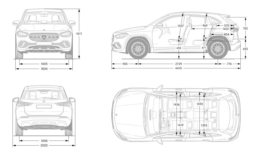
All figures in millimetres. The illustrated dimensions are mean values. They are valid for vehicles in basic specification and in unladen condition.
