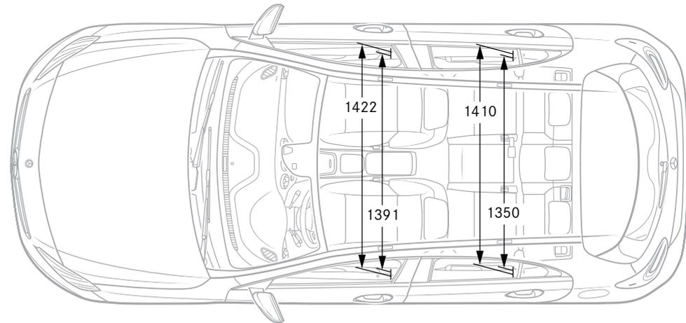
All dimensions in millimetres. The dimensions shown are mean values and apply to standard-specification, unladen vehicles.
