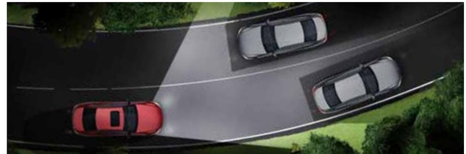
The **MULTIBEAM LED headlamps** react quickly to the current road and traffic conditions with individually controllable LEDs. The partial main beam masks out other road users detected; when the road ahead is clear, **ULTRA RANGE Highbeam** switches to permanent long-range illumination of the carriageway.
