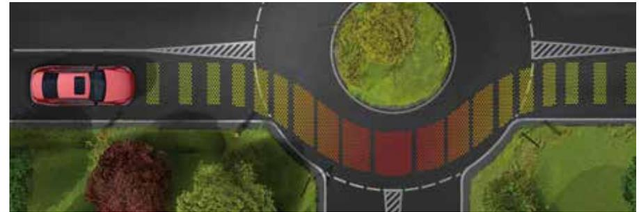
**Route-based speed adaptation** anticipates upcoming road features such as bends, junctions or roundabouts and adjusts the vehicle's speed accordingly.
