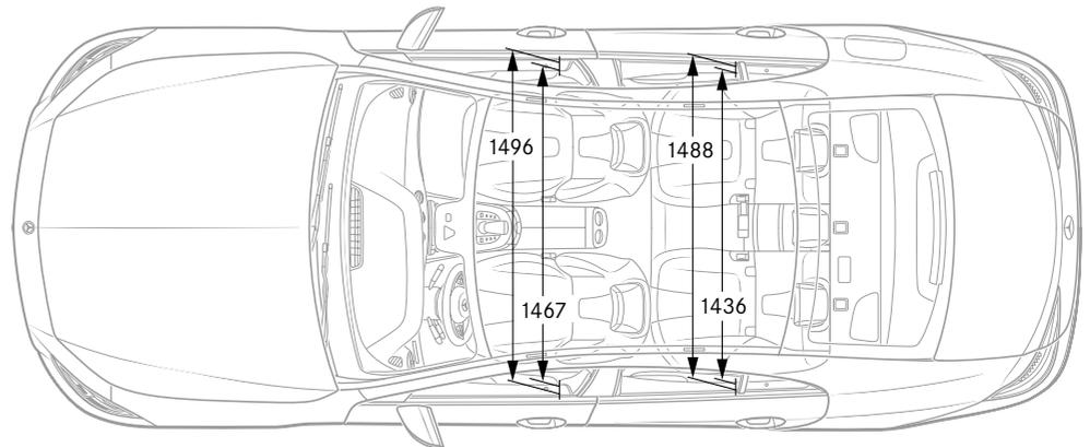
All figures in millimetres. The dimensions shown are median values. They are applicable for unladen vehicles in the standard specification.
