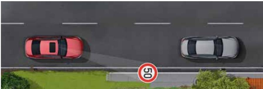
**Active Speed Limit Assist** adopts speed limits detected by camera or known to the navigation system as the new set speed for **Active Distance Assist DISTRONIC**.
