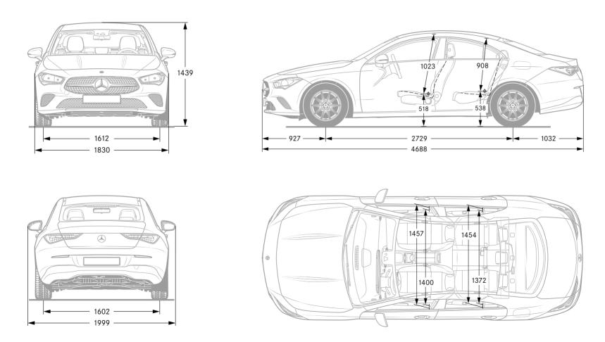
All figures in millimetres. The illustrated dimensions are mean values. They are valid for vehicles in basic specification and in unladen condition.
