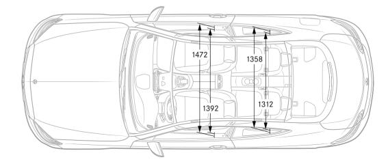
All figures in millimetres. The dimensions shown are mean values and apply to standard-specification, unladen vehicles.
