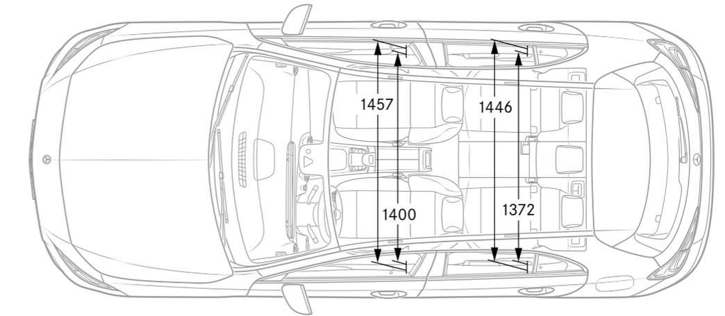
All figures in millimetres. The dimensions shown are average values. They are valid for vehicles in basic specification and in unladen condition.
